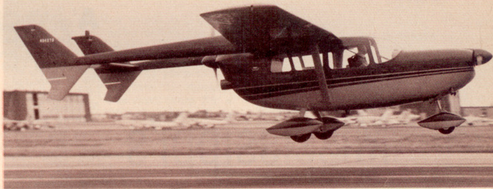
Here is the Cessna Skymaster as it took off at Wichita on its first flight. Note engines at front and rear of cabin section, which Cessna says will assure greater safety for single-engine operation
